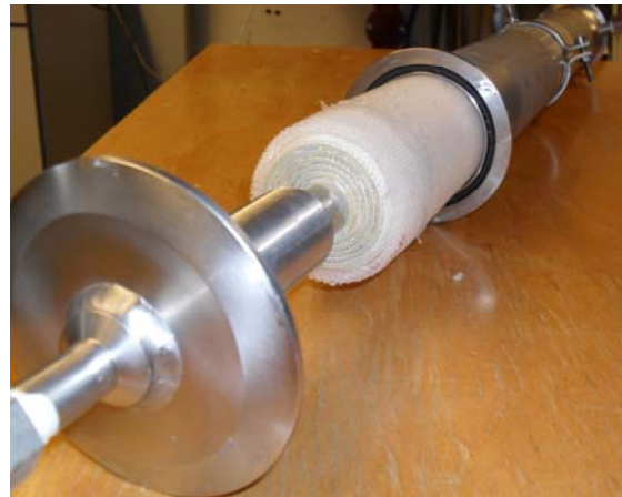
Figure WP3.3 Influence of pH on mass transfer (a) and a photograph of one of the tested membrane elements.
